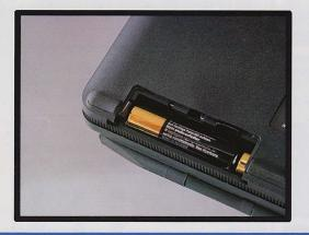
**Power Supply.** The Portfolio is powered by three alkaline AA batteries (batteries included). Or, you can conserve battery power by using an AC adaptor. Since peripherals take their power from the Portfolio's batteries or AC adaptor, they do not need their own power sources.
