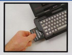
**Memory Cards.** The Portfolio stores and retrieves data and programs from credit card sized memory cards inserted into the built-in card drive, just like floppy disks on a desktop computer. Memory cards are available in three sizes, 32K, 64K, and 128K to provide the right amount of storage for your needs. The card drive also accepts program cards, which can contain commercial software or custom programs.
